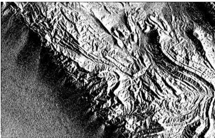
Figure 11. Ravar Terrain Aspect Map: Aspect map generated from the 10 m DEM of the Ravar study area. This morphometric layer captures slope direction patterns and provides supporting terrain characterization for geomorphological interpretation.
