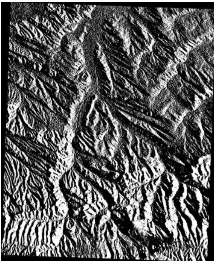
Figure 8. Moghan Terrain Aspect Map: Aspect map extracted from the 10 m DEM for the Moghan region. This layer describes the directional orientation of terrain slopes and was used as an auxiliary morphometric descriptor within the expanded modeling experiments.
