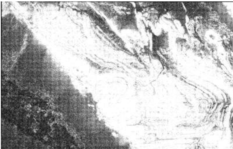
Figure 16. Ravar TRI Map: TRI raster for the Ravar region, representing local elevation heterogeneity and micro-topographic roughness. This index provides strong explanatory power in both baseline and machine learning K prediction stages.
