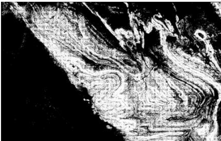
Figure 13. Ravar Hybrid K Coefficient Map (K_Hybrid): Final hybrid K coefficient prediction for the Ravar region, generated using the trained machine learning model integrating slope, TRI, NDVI, and Sentinel-1 VV radar backscatter. The resulting raster represents a continuous K score capturing both geomorphometric and environmental controls.
