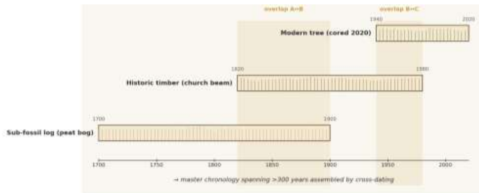
Figure 4.2 · The cross-dating principle. The ring-width sequence of a living tree can be matched to that of progressively older historical and archaeological timbers, extending the absolute chronology centuries or millennia into the past.
