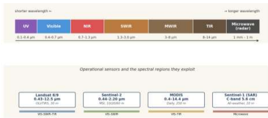
Figure 6.1 · The electromagnetic spectrum and the ranges sampled by common Earth-observation sensors. Optical sensors (Landsat, Sentinel-2) operate in the visible, near-infrared (NIR) and shortwave-infrared (SWIR); thermal sensors operate in the mid- and long-wave infrared; LiDAR uses a narrow band in the NIR; synthetic-aperture radar (SAR) such as Sentinel-1 operates at microwave wavelengths.
