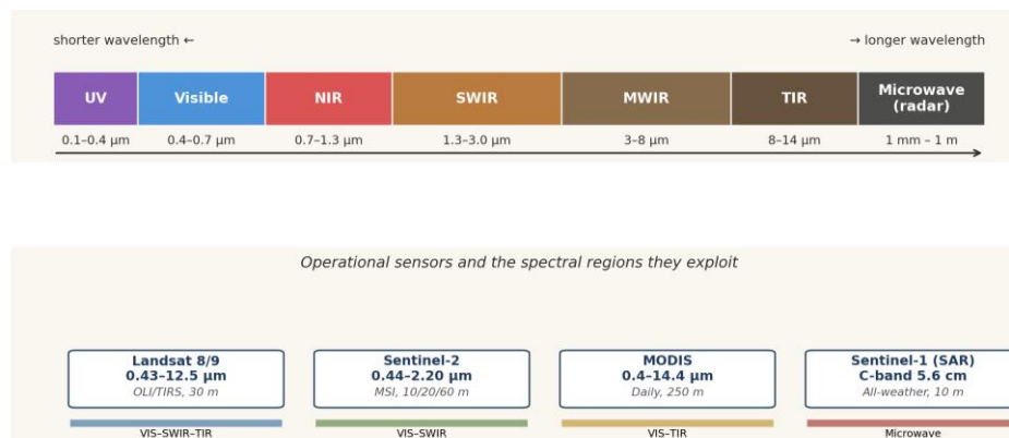
Figure 6.1 · The electromagnetic spectrum and the ranges sampled by common Earth-observation sensors. Optical sensors (Landsat, Sentinel-2) operate in the visible, near-infrared (NIR) and shortwave-infrared (SWIR); thermal sensors operate in the mid- and long-wave infrared; LiDAR uses a narrow band in the NIR; synthetic-aperture radar (SAR) such as Sentinel-1 operates at microwave wavelengths.
