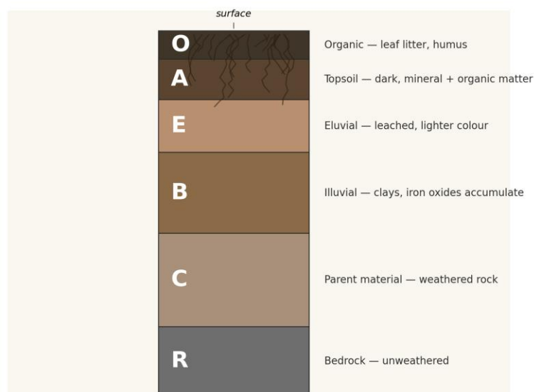
Figure 2.2 · Idealized soil profile and horizon nomenclature. The depth of each horizon and the contrast between them depend on climate, parent material and the amount of time that has elapsed since the surface stabilized. In dry climates, soils may be only weakly differentiated; in humid temperate climates, the contrasts can be very strong.
