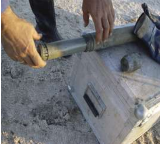
Figure 4- core sampling of the drilling
