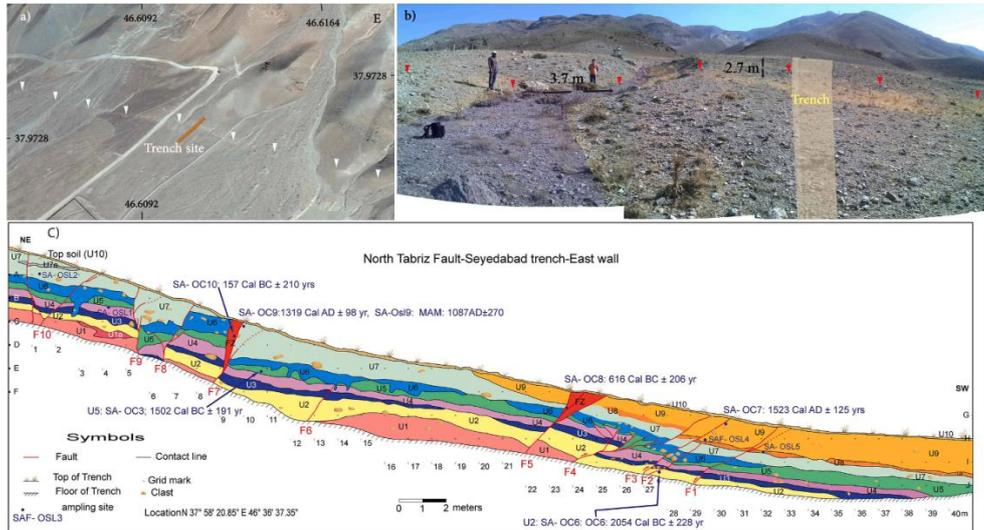
Figure 3: a: Trace of NTF and location of Seydabad trench on Google image; b: Fault scarp and deflected drainage nearby the trench site; c: Trench log showing the sedimentary units (U1 to U10) displaced by fault planes (F1 to F10), sampling points and calibrated ages of the units are given in AD calendar. A, B and C on vertical axis have 1 m intervals. Re-stored sections are illustrated in Supplementary Materials.
