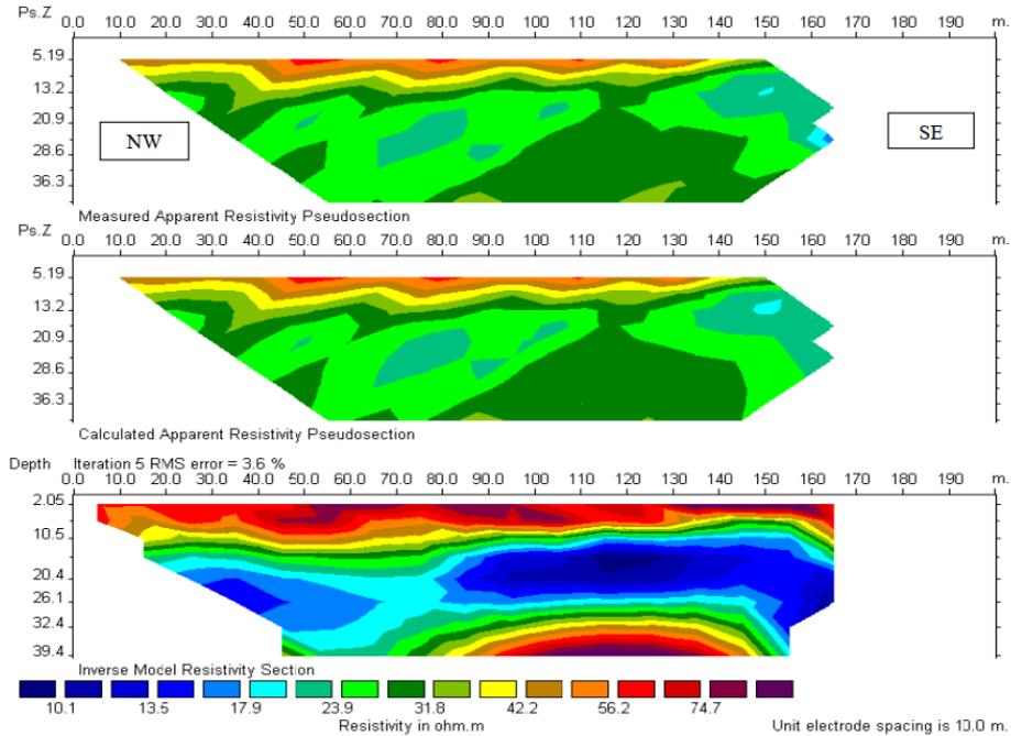
Figure 11: True resistivity pseudo-section together with model, profile one (pole-dipole array).
