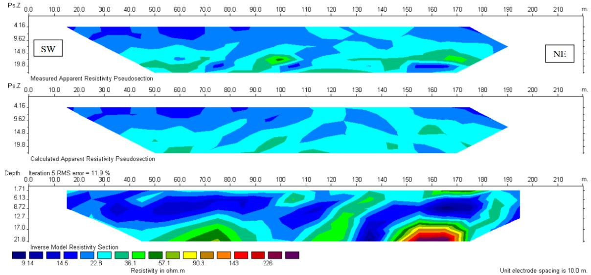
Figure 19: Modelled true-resistivity pseudo-section, profile three.
