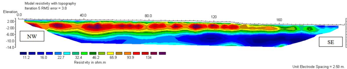
Figure 14: Modelled true-resistivity sections by applying topographical correction on profile one (Wenner array).
