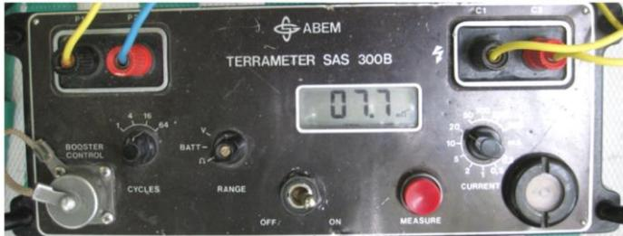
Figure 8: Resistivity terrameter SAS300B apparatus (Swedish)
