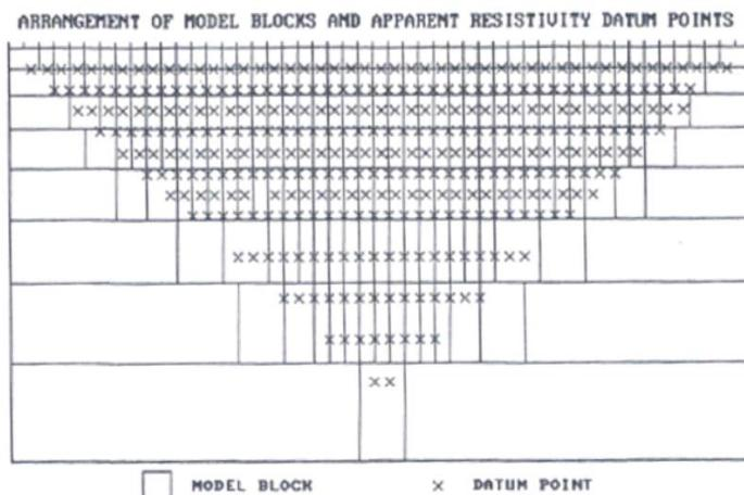
Figure 7: The position of the blocks used in the model relative to the survey points in the pseudo-section.
