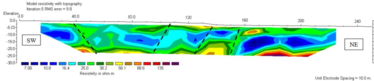
Figure 18: Modelled true-resistivity sections with topographical correction.
