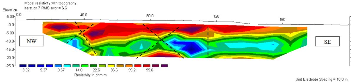
Figure 10: Modelled true resistivity sections by applying topography correction on profile one (dipole-dipole layout).
