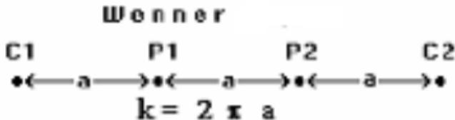
Figure 4: The arrangement of the electrodes in the wenner array.
