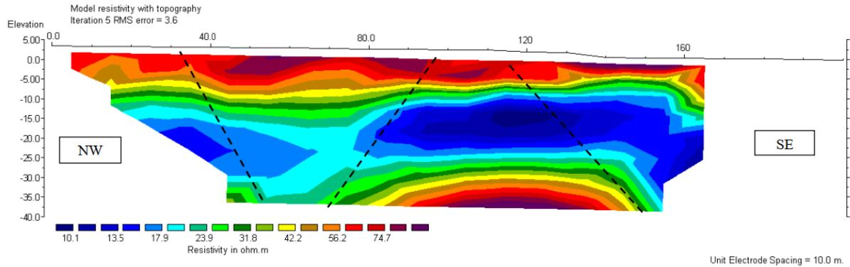
Figure 12: Modelled true-resistivity sections by applying topographical correction on profile one (pole-dipole array).
