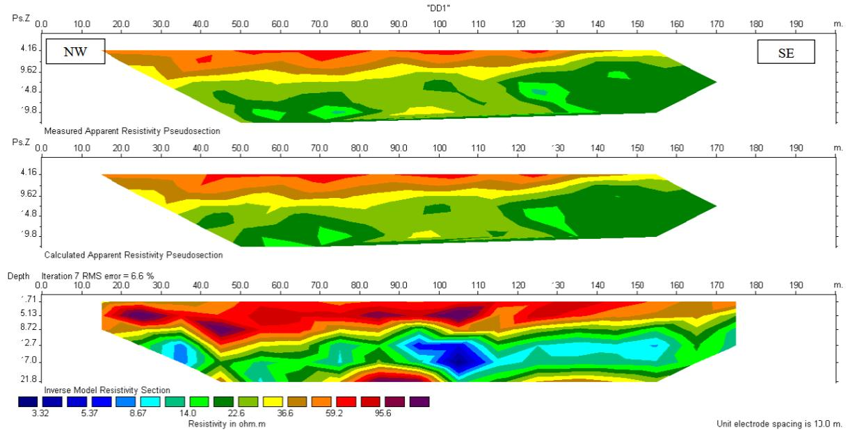
Figure 9: Pseudo-section of true resistivity along with model, profile one.
