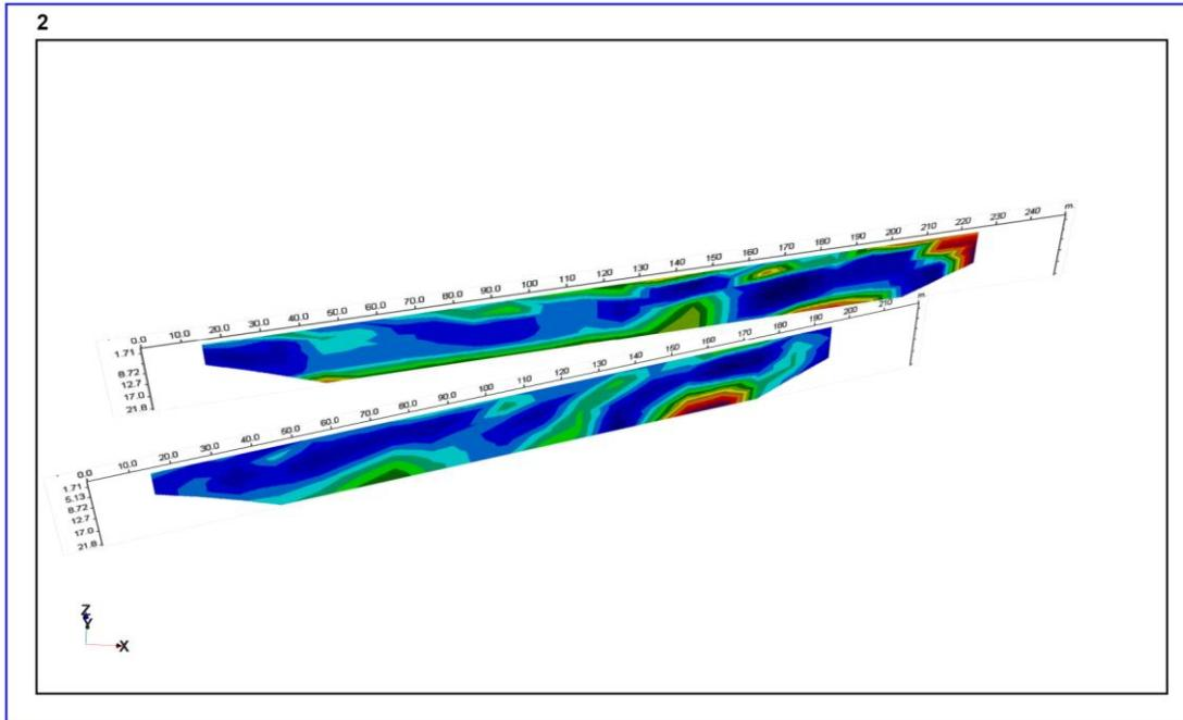
Figure 21: 3D image of modelled true-resistivity sections of profiles two and three.
