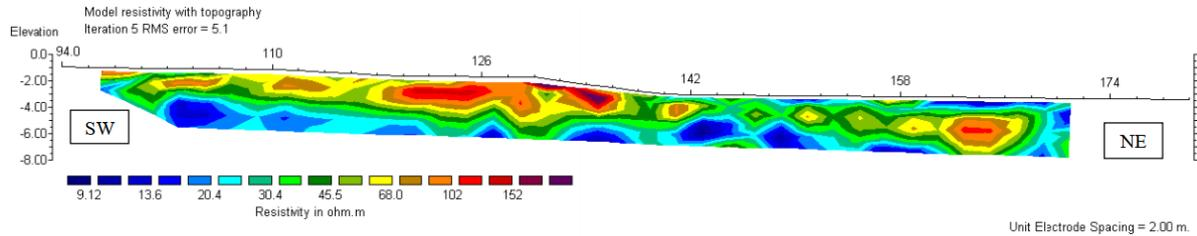
Figure 16: Modelled true-resistivity sections with topographic correction (with 2 m station intervals).
