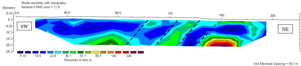
Figure 20: Modelled true-resistivity sections by applying topography correction on profile three.
