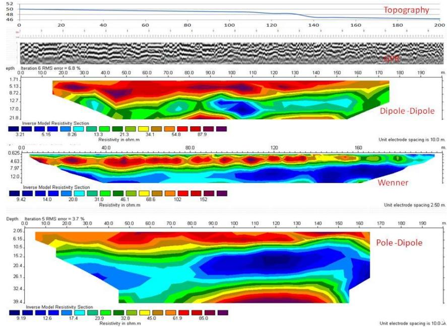
Figure 15: Modelled true-resistivity sections with three different arrays together with GPR section, in profile one.
