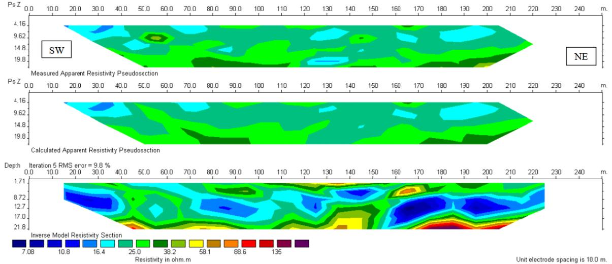
Figure 17: True-resistivity pseudo-sections along with the model (with 10 m station intervals).
