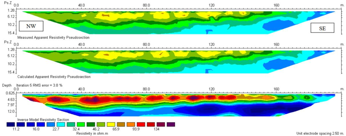
Figure 13: Modelled true-resistivity pseudo-section, profile one (wenner array).
