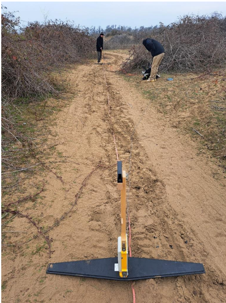
Figure 17: CMP surveying for wave speed analysis using 100 MHz unshielded antenna at station 1330 along profile 2.
