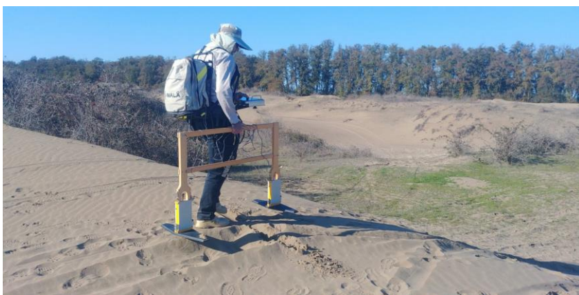
Figure 16: GPR data surveying with 200 MHz unshielded antenna along profile 1.
