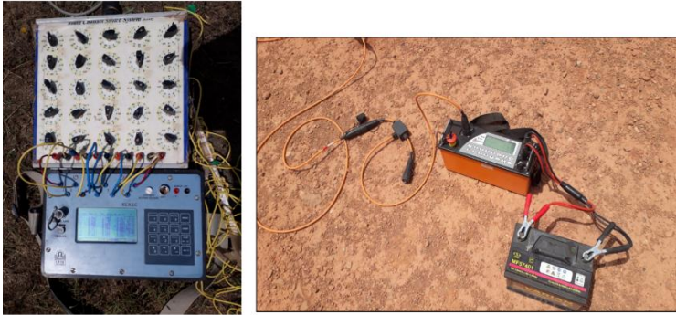
Figure 11: ARES device and related cables, with ELREC-10 receiver.
