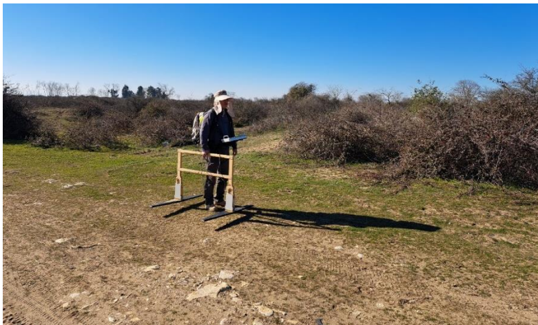
Figure 15: GPR data surveying with 100 MHz unshielded antenna along profile 1.
