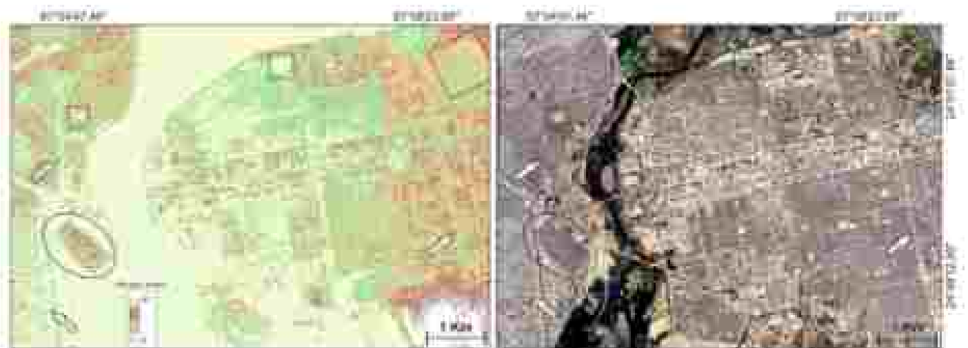
Fig. 4 A comparison of the DTM (left) and a satellite image (right) of a section of Karachi. The buildings in the 3D view show the building structures as compared with the ground conditions in the surroundings. The arrow and circular points in the 3D view indicate the sites (black, open circle) in between the densely populated areas used for the DTM interpolation.
